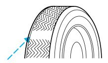
When replacing full size tires, never mix radial bias-belted, or bias-type tires. Use only the tire sizes that are listed on the Certification Label. Make sure that all tires are the same size, speed rating, and load-carrying capacity. Use only the tire combinations recommended on the label. If you do not follow these precautions, your vehicle may not drive properly and safely.
